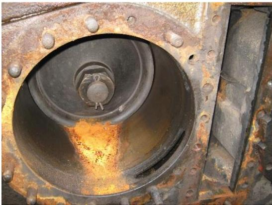
Some items have had to be removed from the locomotive to allow corrosion to be treated. On 5 February the pistons were removed from the bores after many hours struggling to break the rust's hold on the crossheads.
