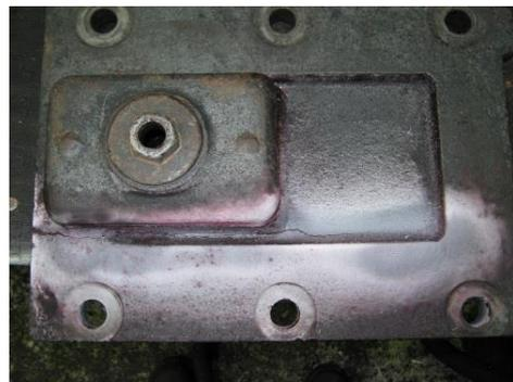
The replacement part required overhauling, including white metalling and machining to suit. New side slipper blocks required manufacturing and shims fitting.
